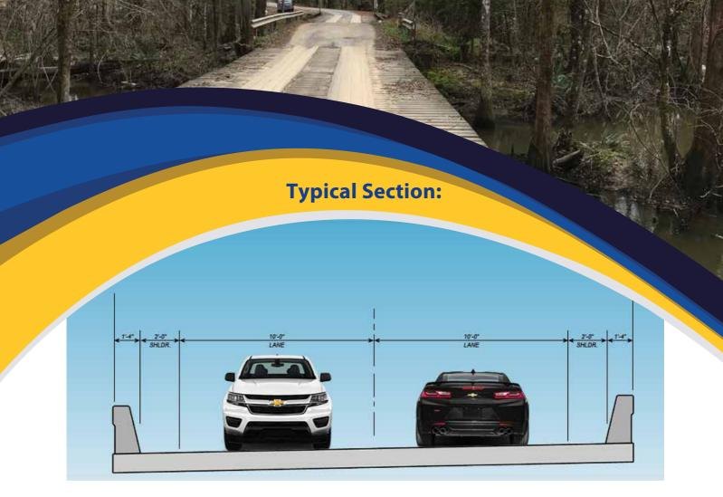
The two-lane concrete bridge will provide a ten-foot wide travel lane with a two-foot wide shoulder in each direction.
